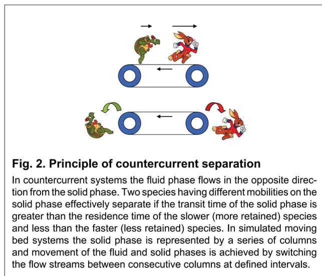
**Fig. 2. Principle of countercurrent separation**
